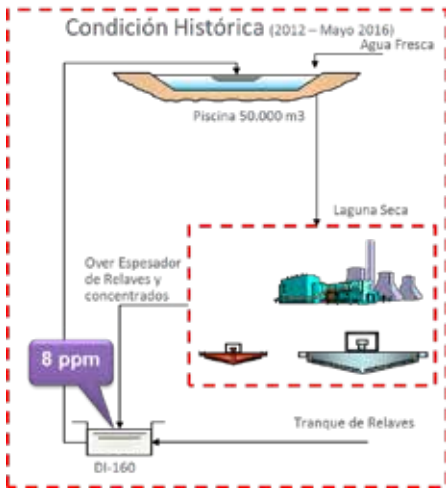
Process water system before optimization
